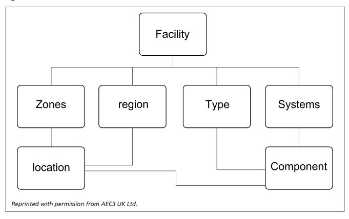
For buildings, the assets include the Facility as a whole and its constituent Spaces and Components. These are managed through groupings into Zones, Floors, Types and Systems (see Figure 4).
