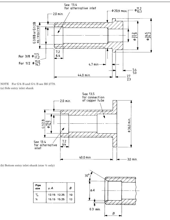
(c) Inlet (bottom or side entry) for connection to 12 mm or 15 mm copper tube (see clause **13.4**) All dimensions are in millimetres.
