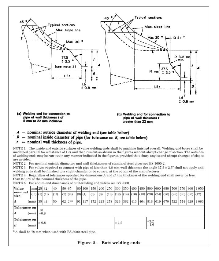
**8.7** Butt-welding ends shall comply with the details shown in Figure 2.
