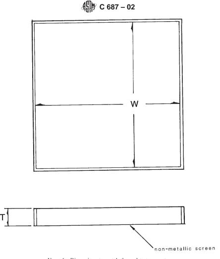
NOTE 1—Dimensions to match thermal test apparatus. FIG. 1 Rigid Test Frame
