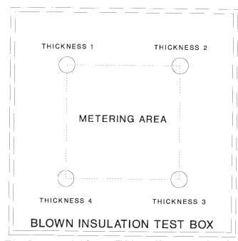
FIG. 4 Recommended Contact Thickness Measurement Locations
