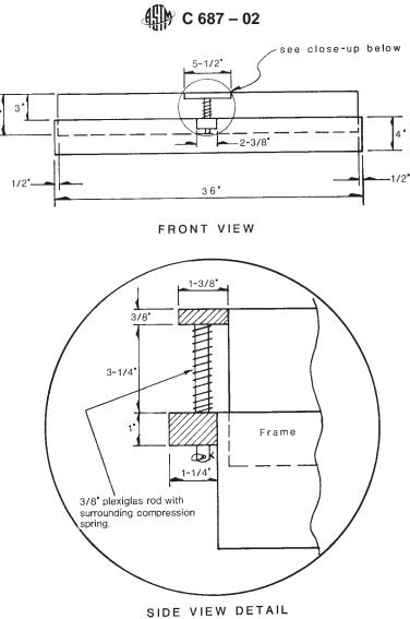
FIG. 2 Collapsible Test Frame (an Example)
