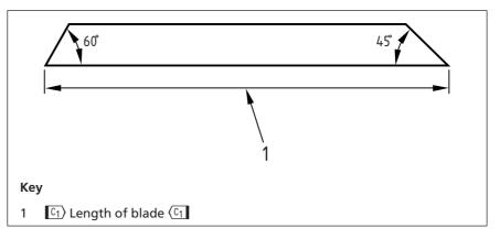
NOTE The thickness of 4.8 mm<sup>13</sup>/<sub>16</sub> in for mechanical types has been adopted to accommodate the present practice of manufacturers but it is desirable that the minimum thickness should be 6 mm<sup>11</sup>/<sub>4</sub> in.
