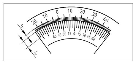
Figure 6 Section through scale and vernier
