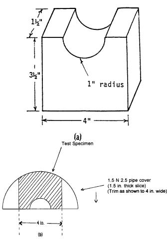
FIG. 5 Insulation Test Block Dimensions and Groove Location
