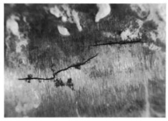
FIG. 2 Typical External Stress Corrosion Cracks (5 $\times$  Magnification)
