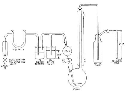
FIG. 4 Sulfur Distillation Apparatus
