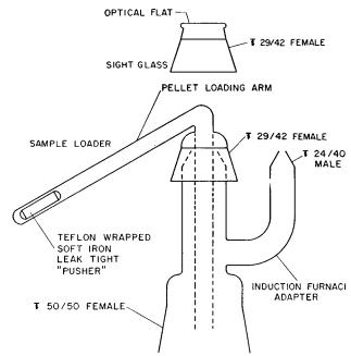
FIG. 7 Furnace Tube Adapter and Sample Loader
