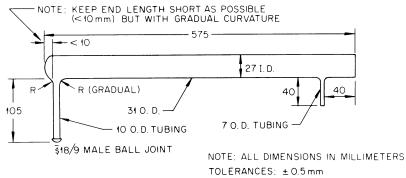
FIG. 2 Quartz Reaction Tube
