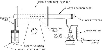
FIG. 3 Pyrohydrolysis Apparatus
