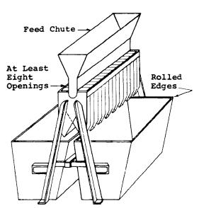
FIG. 1 Large Sample Splitter for Coarse Aggregate
