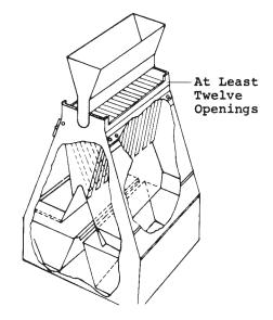
Note— Small Sample Splitters for Fine Aggregate. May be constructed as either closed or open type. Closed type is preferred. FIG. 2 Sample Splitters (Riffles)
