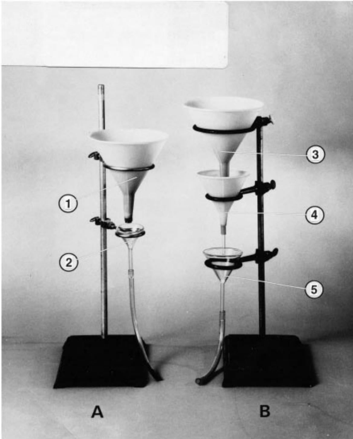
NOTE 1—Identified by number in this figure are: (1) main supply funnel with metering insert, (2) gun supply funnel, (3) main supply funnel, (4) metering funnel, and (5) gun supply funnel.
