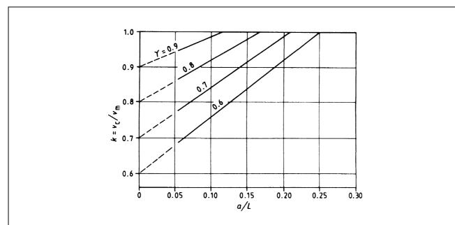
Figure 4 — Influence of steel reinforcement on pulse velocity: correction factors for bars parallel to pulse path (a > 2 b) [see Figure 3 a)]
