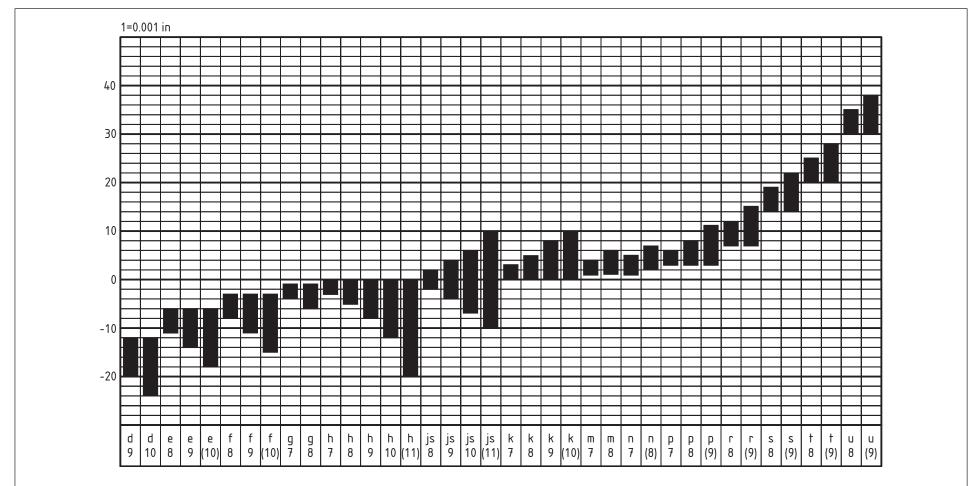
NOTE Diagram to scale for diameters 24.81 in to 27.96 in.
