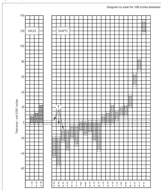
NOTE The diagram illustrates the effect of errors of measurement on the actual limits if no safety zone is introduced.
