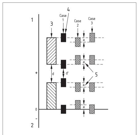
CASE 1. No safety zone. The limits can vary by amount of error of measurement. Actual deviation "d" can become d' where d-d' = 2 × 30 microinches per inch.
