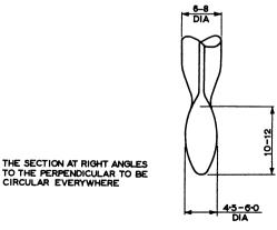
Fig. 1. Bulb of 'congealing point' thermometer.
