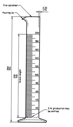
Shape of foot optional; cylinder must stand on 15° slope without tipping
