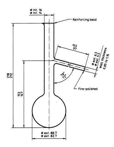
Figure A.1 — 250 ml distillation flask
