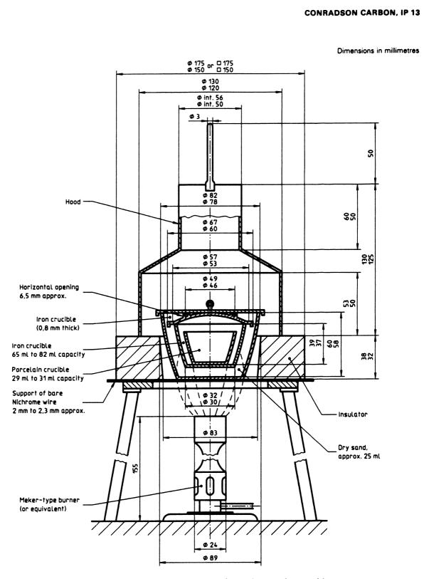
Figure 1 — Apparatus for determining Conradson carbon residue
