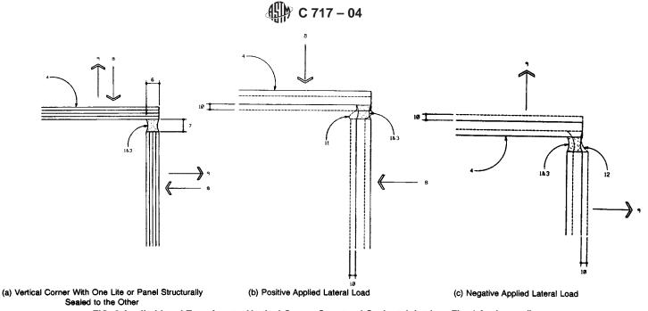
FIG. 2 Applied Load Transfer at a Vertical Corner Structural Sealant Joint (see Fig. 1 for Legend)
