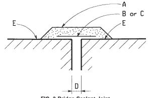
FIG. 3 Bridge Sealant Joint
