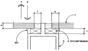
(c) Structural Sealant Joint to the Edge and Face of a Lite or Panel
