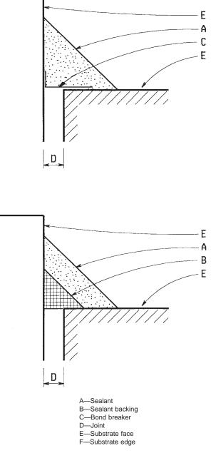
FIG. 5 Fillet Sealant Joints
