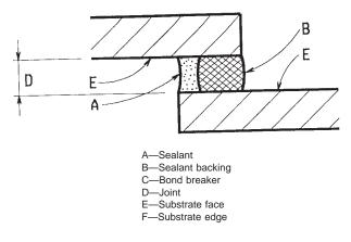
FIG. 6 Lap Sealant Joints
