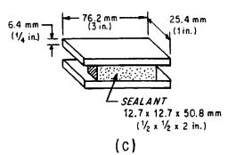
FIG. 1 Preparation of Test Specimen
