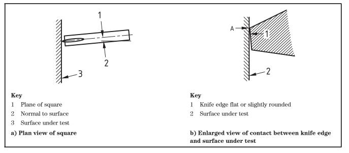
If the sharp edge, A, formed by the junction of the bevel and the reduced edge of the blade is not straight and/or laterally parallel to the plane of the square, the square will show erroneous results unless it is presented to the surface under test with its plane truly normal to that surface.
