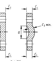
Grey iron blank flanges are supplied flat up to DN 200 and dished or domed for DN 250 and greater. Ductile iron blank flanges are supplied flat up to DN 200 and optionally flat, dished or domed for DN 250 and greater. The face is permitted to be either on the concave or convex side of dished blank flanges.
