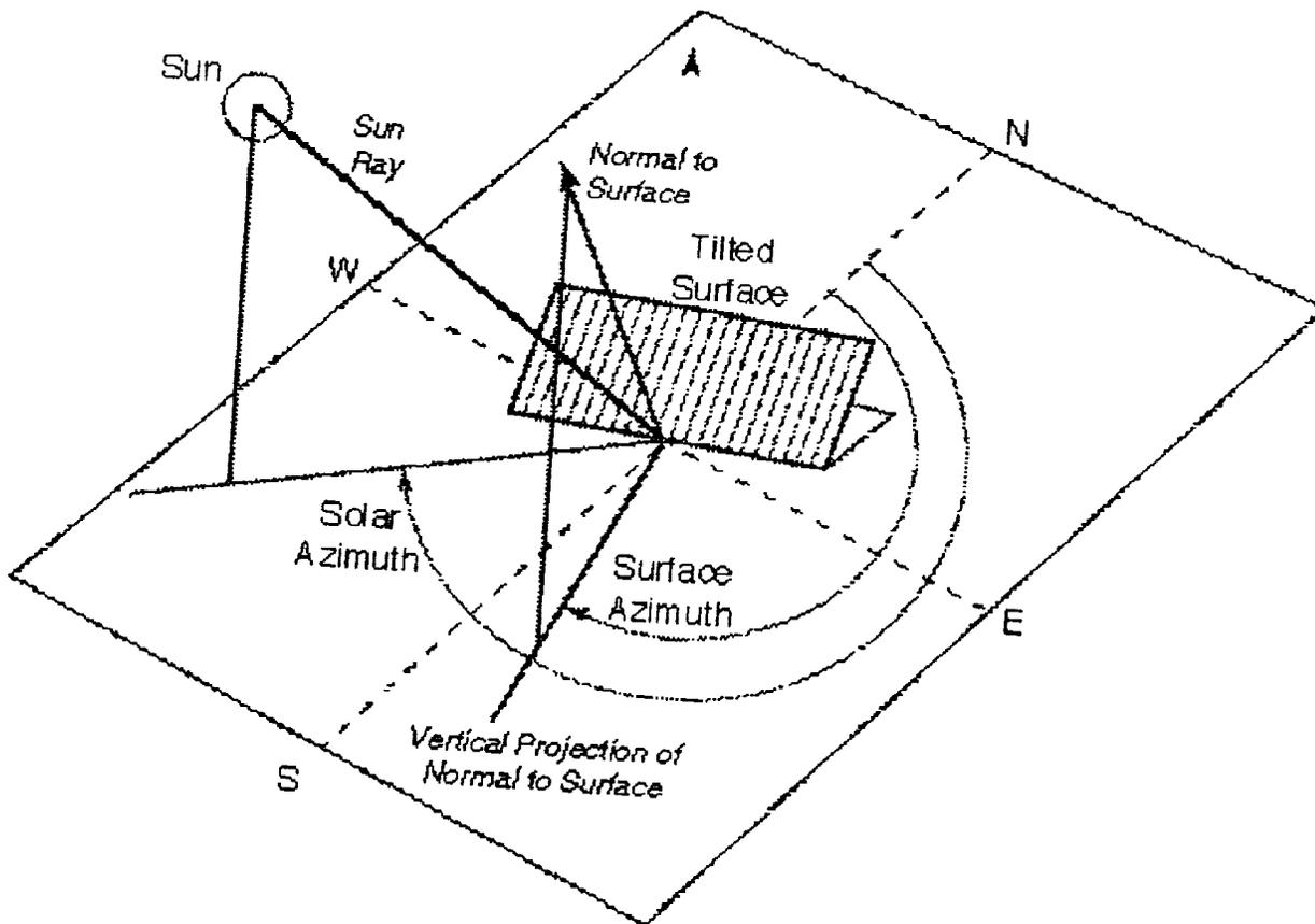
FIG. 1 Solar Azimuth Angle
