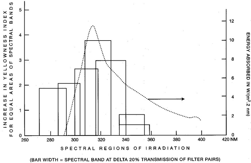
FIG. X1.4 Activation Spectrum of Yellowing of 2 mil Polysulfone Film Exposed Behind Sharp Cut-On Filters to Xenon Arc Radiation Through Daylight Type Filters Compared with the Spectral Energy Absorbed by the Polymer
